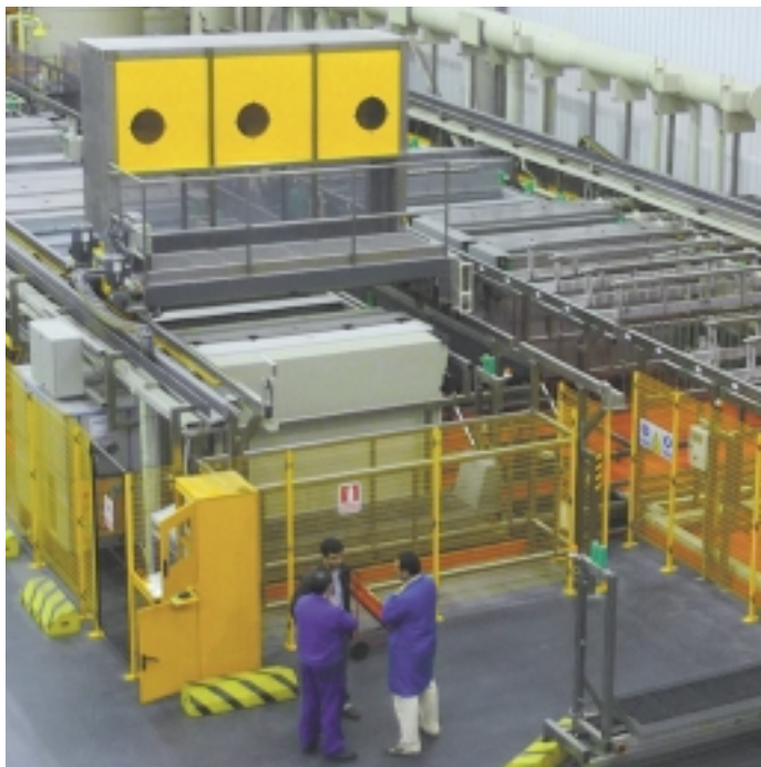
AHC Full automatic installation for a chemical nickel process, free of lead (Durni-Coat®)
