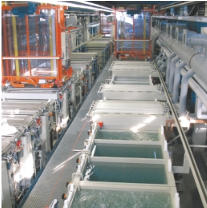
Traterh HART-COAT® process for hard anodising of aluminium alloys
